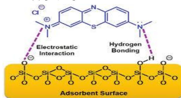
Scheme 1 :Represent the interaction between methylene blue and MCM-41.
