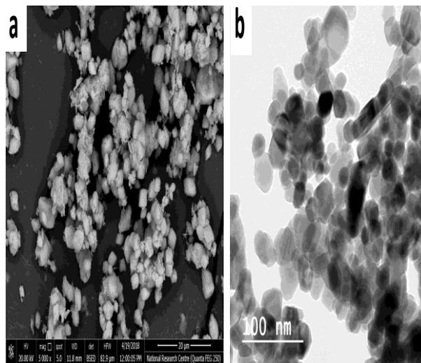
**Figure 2** – a and b are the FE-SEM and HR-TEM images of ZnO respectively
