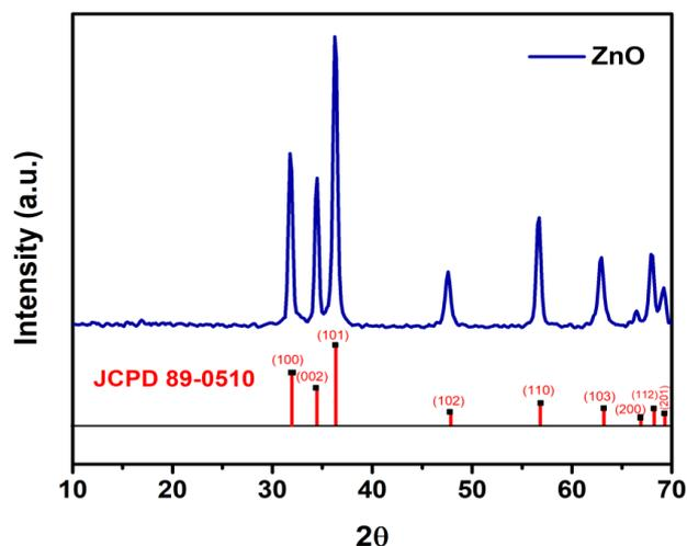
**Figure 1** – X-ray diffraction pattern of ZnO.
