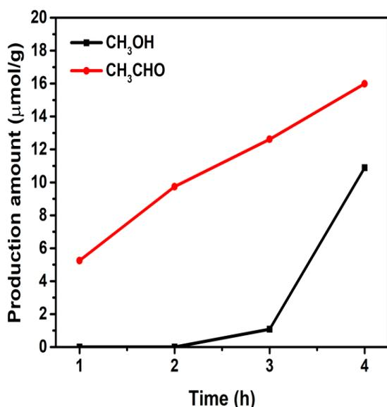
**Figure 3** - Production yield over ZnO in 0.5 M a)  $\text{NaHCO}_3$ , b)  $\text{NaOH}$ , and c)  $\text{NaCl}$  aqueous solutions.
