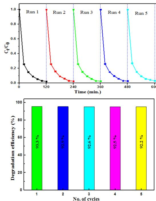
**Fig. (5)** Recycling of CuS-Plu. photocatalyst for degradation of 10 ppm MG dye solution.
