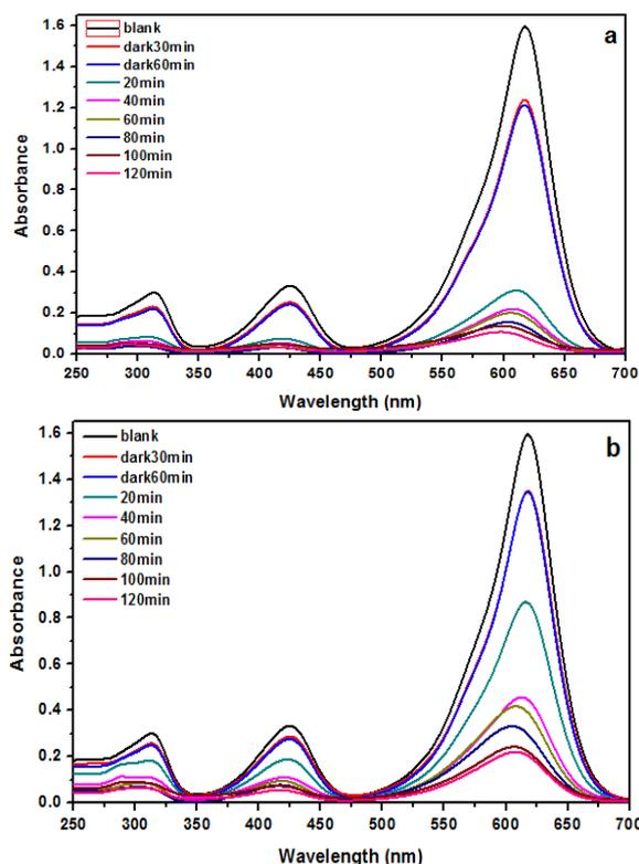
**Fig. (3)** Absorbance spectra of MG with CuS photocatalyst by different surfactant agents (a) Plu. and (b) PVP.
