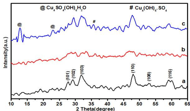
**Fig. (1)** XRD patterns of CuS prepared by using different surfactants (a) Plu.123, (b) PVP and (c) PEG.
