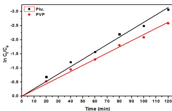
**Fig. (4)** Kinetic study for photodegradation of MG with CuS photocatalyst prepared using different surfactants.
