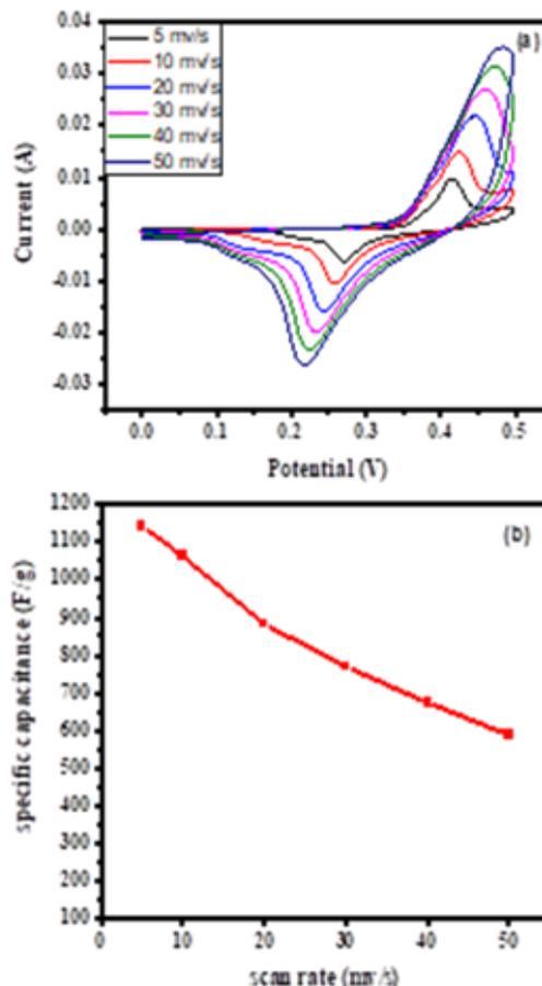
**Fig.3** Cyclic voltammetry curves (a) and (b) specific capacitance as a factor of scan rate of MoS/Ni foam electrode at different scan rate.
