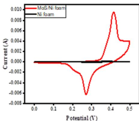
**Fig.2** CV curves of Ni foam supported MoS and pure Ni foam at 5mV/s.
